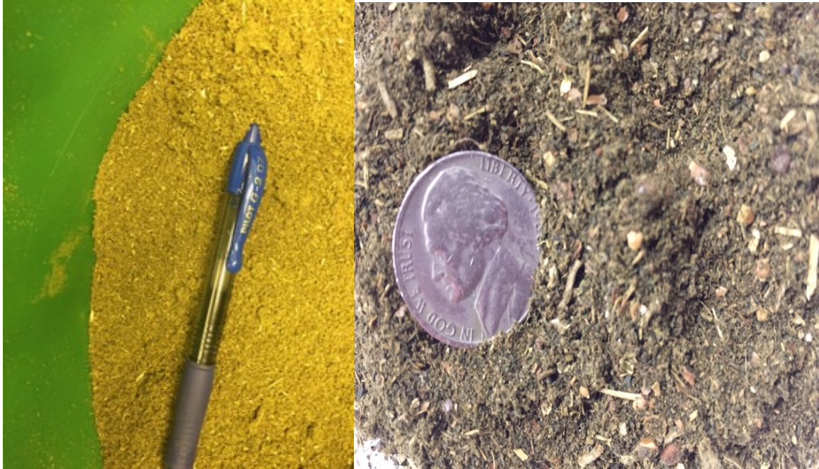
Cannabis Feedstocks That Have Been Ground to ~200micron Size Ready for Processing in the CannabisSFE Unit
