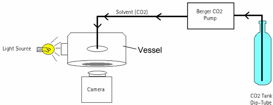
**Figure 1:** General schematic of experimental apparatus, the phase-monitor. Sample would be introduced to the high pressure vessel at various concentrations in the organic modifier volume. Phase monitor modifications were provided through in-house fabrication and control of pressure was accomplished by means of a Berger CO<sub>2</sub> pump. Internal volume of modified vessel is 7 mL.
