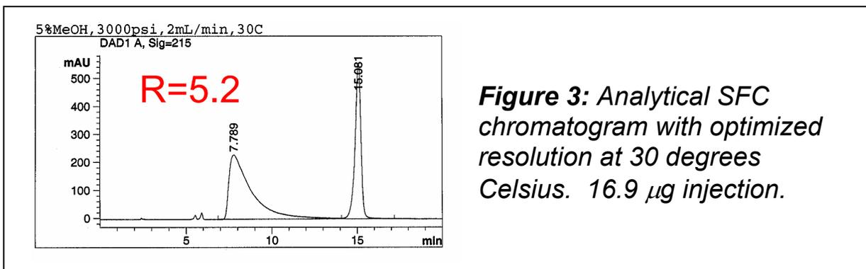
**Figure 3:** Analytical SFC chromatogram with optimized resolution at 30 degrees Celsius. 16.9  $\mu$ g injection.
