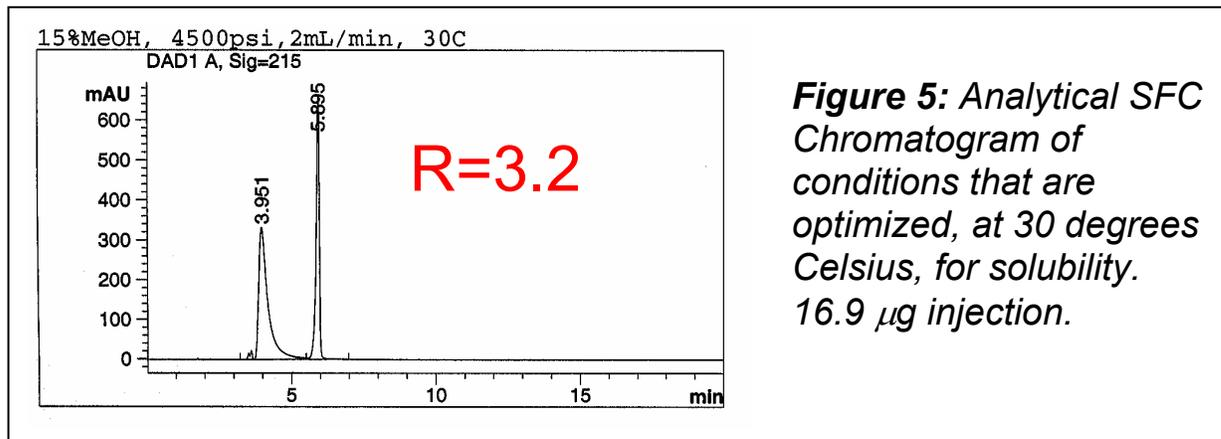
**Figure 5:** Analytical SFC Chromatogram of conditions that are optimized, at 30 degrees Celsius, for solubility. 16.9  $\mu\text{g}$  injection.
