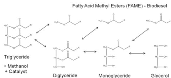
**Figure 2:** Transesterification reaction
