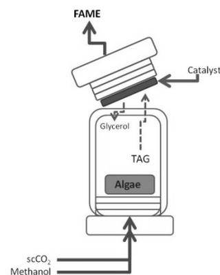
**Figure 6:** Depiction of possible reaction system configuration
