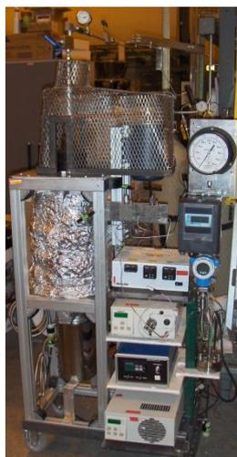
**Figure 1.** High pressure batch reactor system (Digital and Astra gauge, heat control unit for main reactor and pre-heater, HPLC solvent pump, modular mixer speed control, HPLC CO<sub>2</sub> pump)
