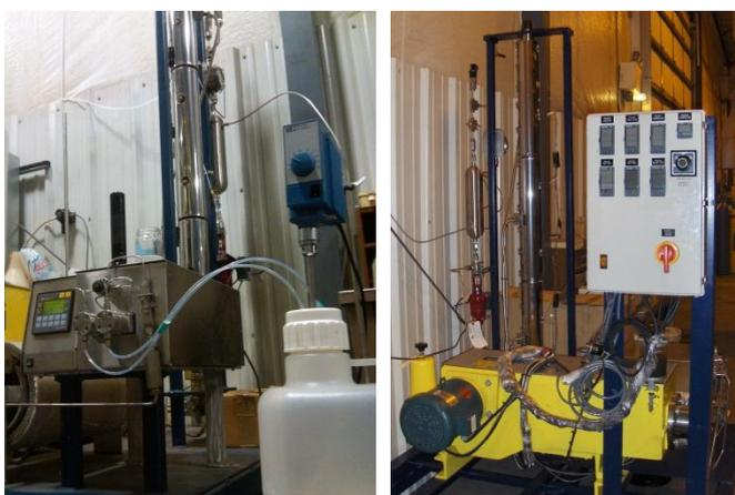
**Figure 2.** Pilot Scale high pressure flow reactor at the Iowa Energy Center-BECON facility
