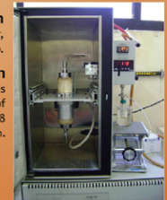
Figure 3. Extraction system SFT-150 by Supercritical Fluid Technology Inc. Newark, U.S.A.
