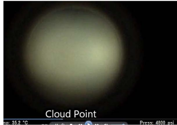
Figure 5. Cloud Point of Benzophenone at 4800 psi
