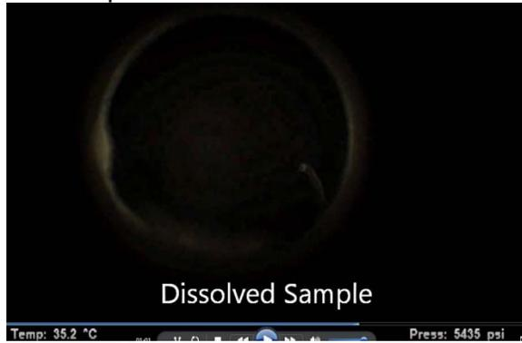
Figure 3. Dissolved Benzophenone Sample at 5435 psi
