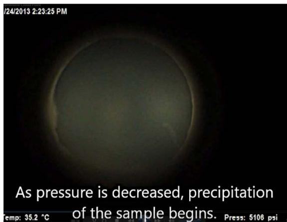
Figure 4. Benzophenone Sample at 5108 psi
